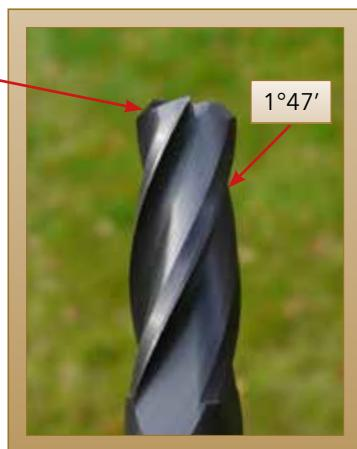
Premilling of conical holes result in longer tool life of thread mill
